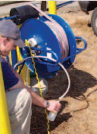
Collecting a water sample from an SVRP aquifer monitoring well.
